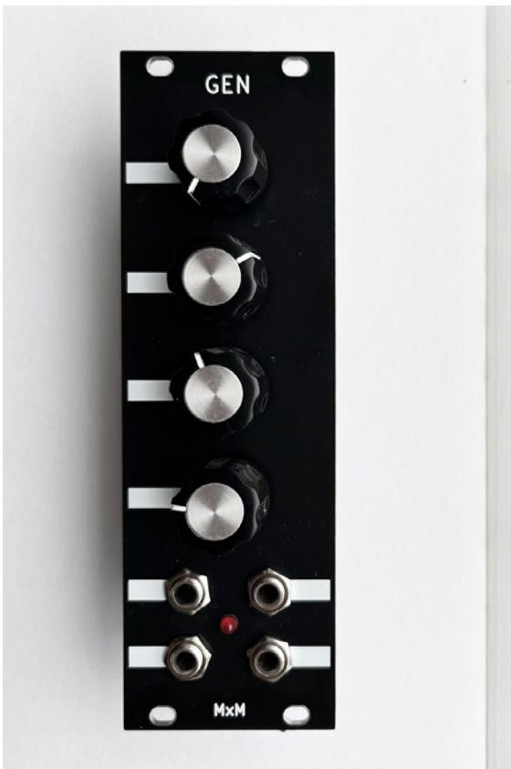
Gen is a generic circuit board and front panel that allows for many different synthesizer modules to be created.
